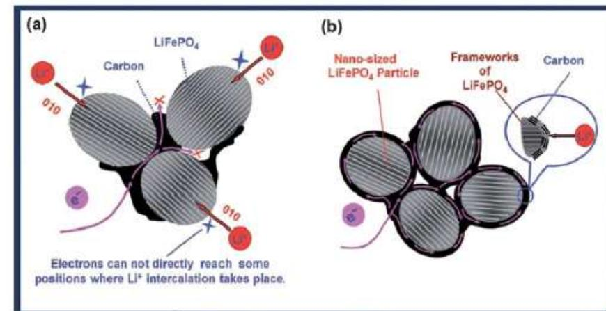
Fig. 4 (a) Electron-transfer pathway for LiFePO<sub>4</sub> particles partially coated with carbon. (b) Designed ideal structure for LiFePO<sub>4</sub> particles with typical nano-size and a complete carbon coating.<sup>58</sup>
