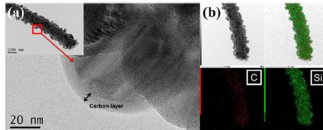
Figure 3. (a) TEM images of carbon-coated Si nanowires. (b) Lower-magnification TEM image and corresponding EDS mapping images of C (red) and Si (green).
