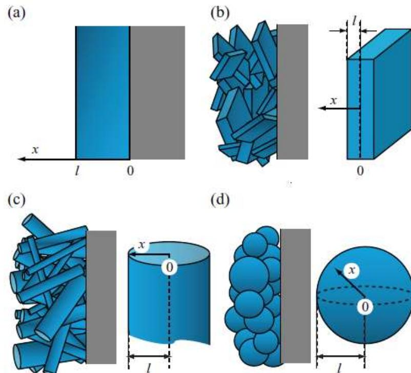
**Figure 1.** Model electrode configurations, particle geometries, and corresponding coordinate systems, where the blue region and the gray region represent the active material and the current collector, respectively: (a) thin film electrode, (b) electrode with planar particles, (c) electrode with cylindrical particles, and (d) electrode with sphere particles.
