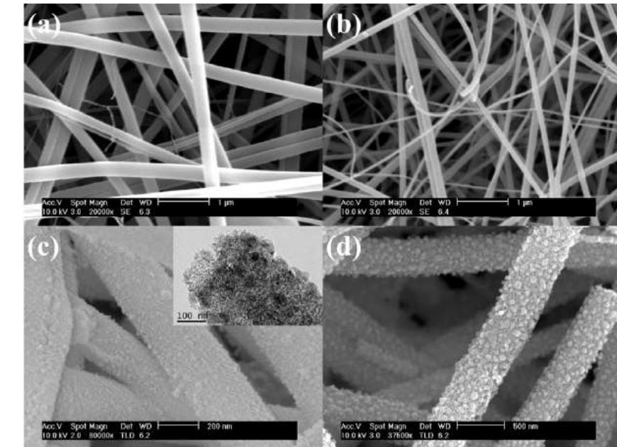
Figure 2. SEM images of (a) as-spun TEOS/PVP nanowires, (b) SiO<sub>2</sub> nanowires after pyrolysis in air, (c) Si nanowires after the Mg reduction and washing steps, and (d) carbon-coated Si nanowires.
