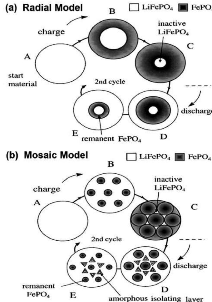
Fig. 3 Schematic models for lithium extraction/reinsertion into a single particle of a LiFePO<sub>4</sub> radial model (a) and Mosaic model (b).<sup>56</sup>
